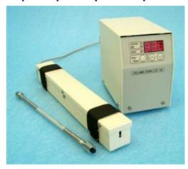
Accurate temperature control of your HPLC columns will **improve the reproducibility of your results**. Operating at increased temperatures provides **better separation performance and reduced analysis time** in most cases. Alternatively, you may need to **chill your columns** when using thermally sensitive compounds. Whatever your requirements, we can supply an HPLC column oven to improve your results!
